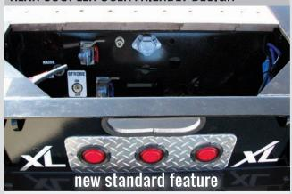
The **rear coupler uses an angled control panel**, making it easier to reach all the needed controls: air, electric, and raise & lower valve.
