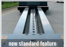
The patented Extend-a-trac now features a **one-piece track pan design** for added stability.
