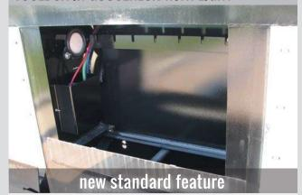
The **lockable toolbox** in the base of the gooseneck has an aluminum cover, a chain rack, and a light to find your items at night with ease.
