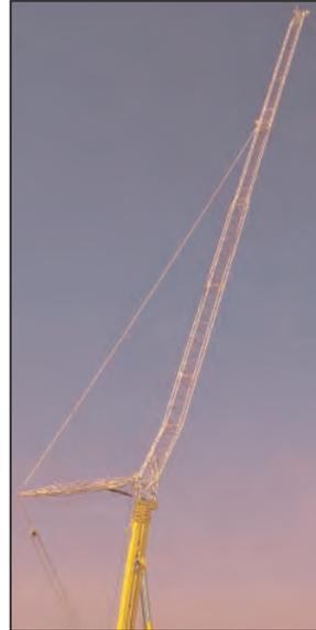
A sturdy 240 ft. (73 m) luffing jib on 179 ft. (54,6 m) of main boom provides up to 410 ft. (125 m) max tip ht with approximately 295 ft. (90 m) of working radius.
