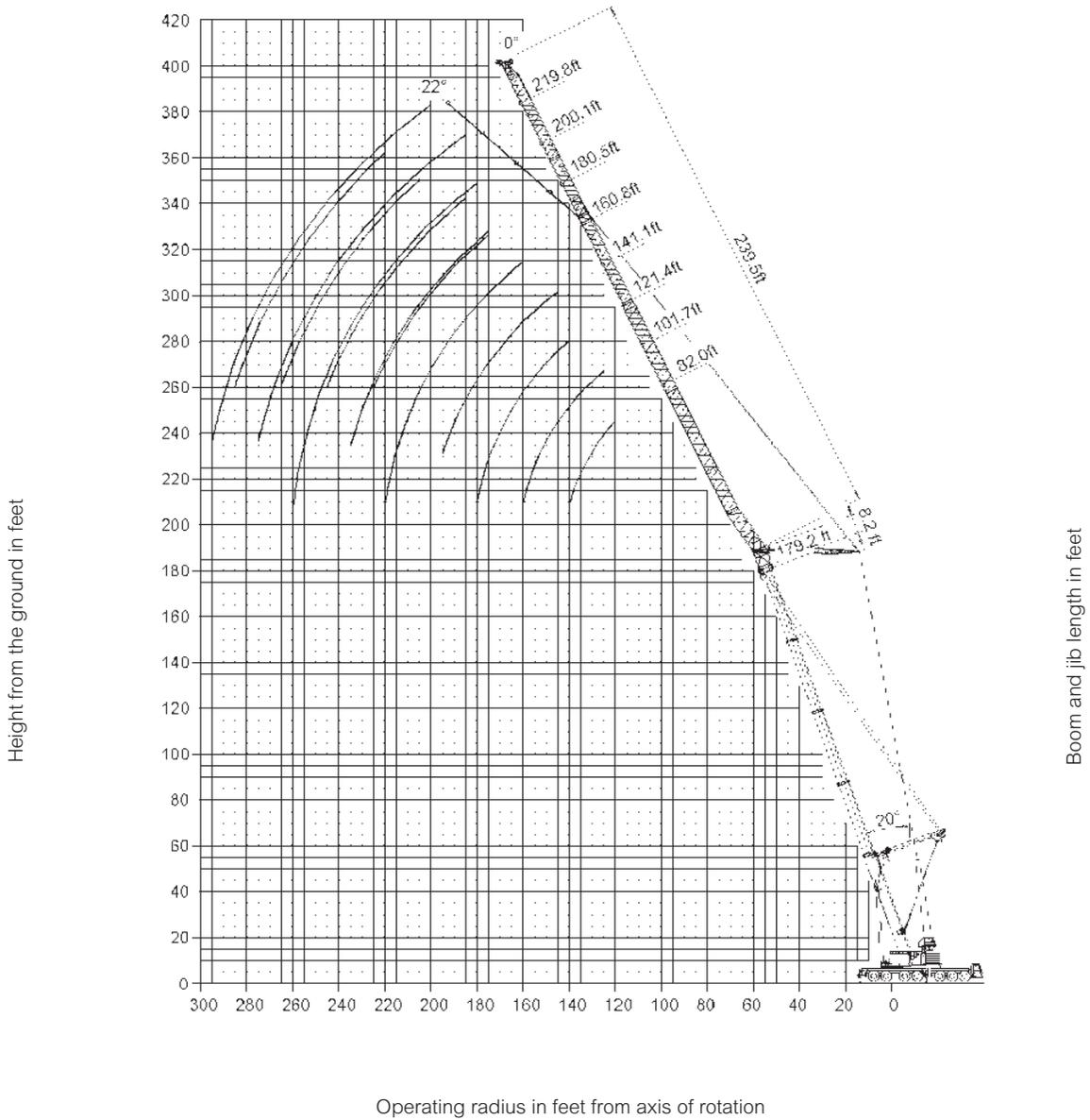
THIS CHART IS ONLY A GUIDE AND SHOULD NOT BE USED TO OPERATE THE CRANE. The individual crane's load chart, operating instructions and other instructional plates must be read and understood prior to operating the crane.
