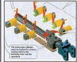
The TWIN-LOCK boom pinning system - a Grove patented design - runs inside a five section MEGAFORM boom.
